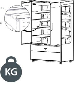
Do not block air vents with product. A minimum of 25mm should be maintained between the top of the product and the shelf above.
