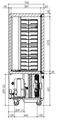
(1) - Evacuation of water from defrost  $\varnothing$ 20 (2) - Electric supply cable
